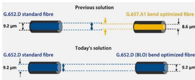
Figure 1: Even when precisely aligned, light is lost when G.652.D is connected to G.657.A1. This no longer happens with the new bend-optimized G.652.D (BLO) fibre.
